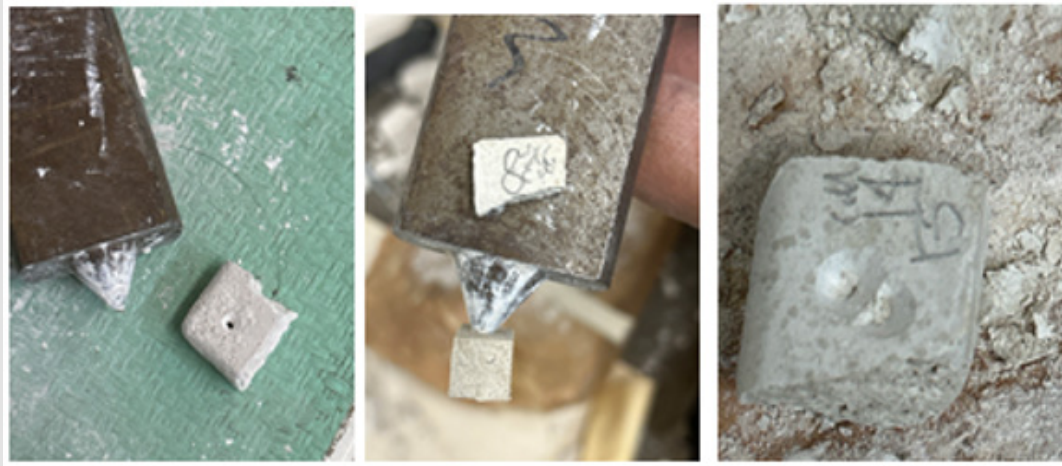
Figure 2: Impact load and tested samples (a-product from gypsum and vinegar solution, b-product from gypsum, water and oil, c-product from gypsum, water and chicken protein).
